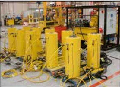
◀ Custom cylinders with embedded sensors for bridge construction.
