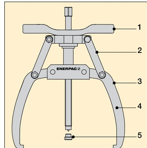
1. Convenient adjustment handle simplifies positioning of jaws on application and increases speed of operation.
