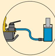
**4-Way Valves** are used with double-acting cylinders
