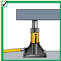
◀ Provide a solid support for the entire cylinder base area. Use cylinder base attachment for more stability.
