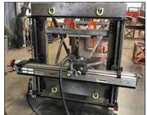
*I-Beam end face milling with a GMRF1000.* ▶
