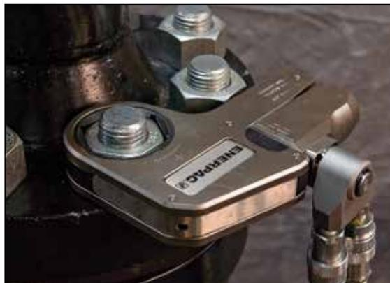
◀ Any brand of hydraulic torque wrench can be powered by the portable ZU4T-Series torque wrench pump.
