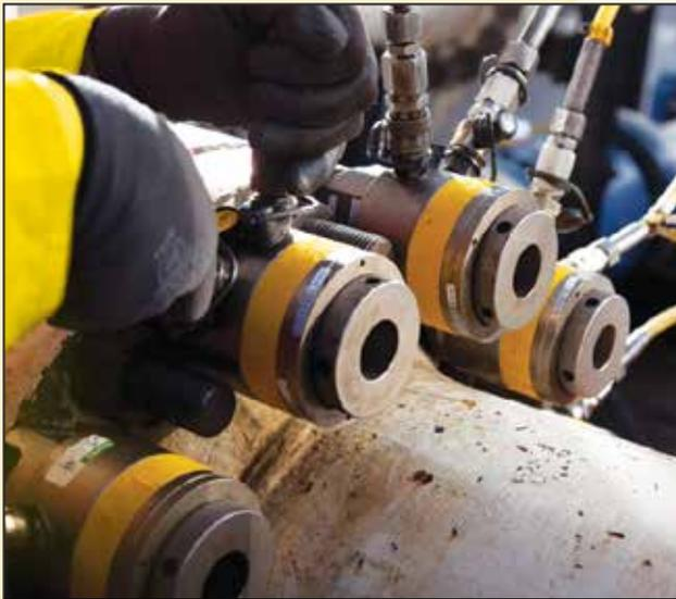
**Safe, reliable, and repeatable tensioning with compact HydraMax® Tensioners to complete joint integrity**
