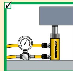
Both couplers must be connected when using double-acting cylinders. Ensure return hose is fitted.
