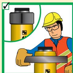
◀ Always protect cylinder threads for use with attachments.
