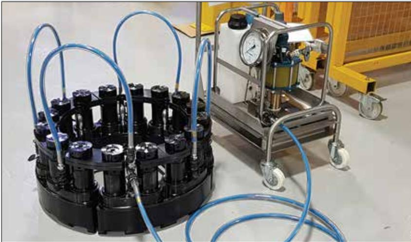
▲ *Multi-Stud Tensioning Set-Up.*
