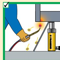
◀ Keep hydraulic equipment away from open fire and temperatures above 150 °F (65 °C).
