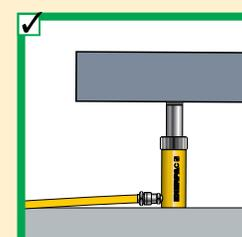
Never allow the cylinder to be lifted off of the ground through the couplers.
