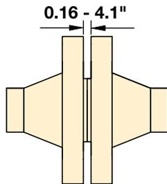
An innovative flange spreading wedge for use on small, medium or large flange joints with a minimum access gap of 0.16 inch. The SWi range includes ATEX approved options.
