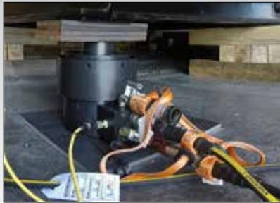
◀ Custom double-acting Lock Nut cylinders with internal stroke sensors and an integrated load holding valve for lifting nuclear components.
