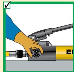
Close release valve finger tight. Using force will ruin the valve.
