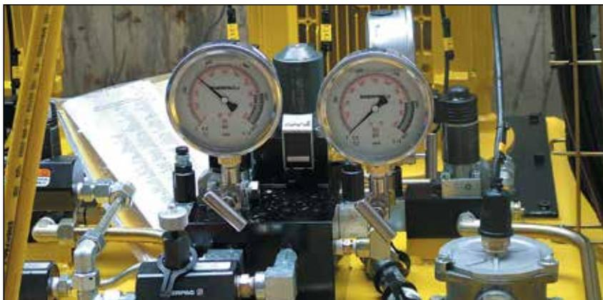
◀ When lifting or pressing, always use a gauge. A gauge is your "window" to the system—it lets you see what's going on.
