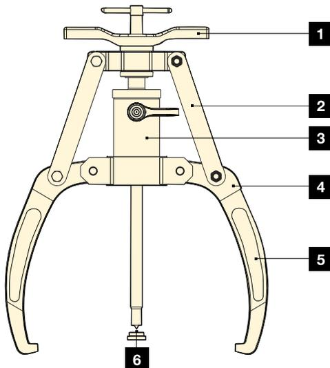
1. Convenient adjustment handle simplifies positioning of jaws on application and increases speed of operation.
