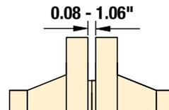
A mechanical tool for small diameter, low pressure flanges with a minimum access gap of 0.08 inch.
