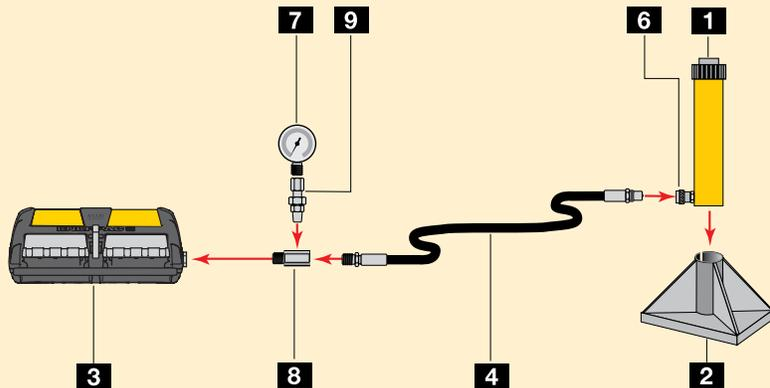
**Double-acting cylinder set-up used for lifting applications where a slow controlled descent of the load must be maintained.**
