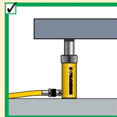
◀ The entire cylinder saddle must be in contact with the load. Movement of the cylinder must be parallel with the movement of the load.
