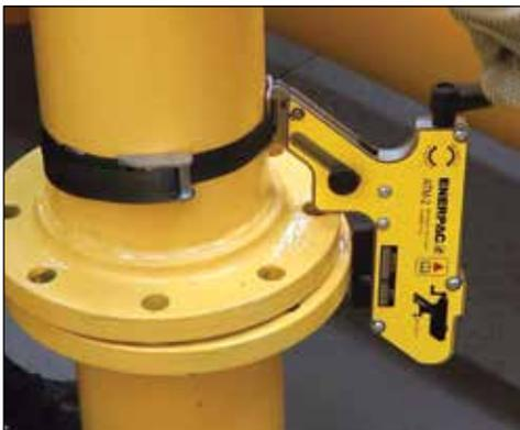
▼ The ATM9 is shown here with optional pressure gauge and gauge adaptor.
