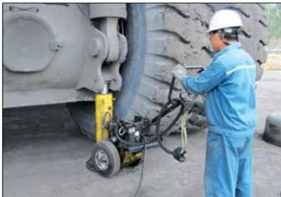
◀ Enerpac POW'R-RISER® used in mining operations to lift heavy equipment.
