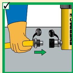
Clean both coupler parts before connecting. Use dust caps when coupler parts are not connected.
