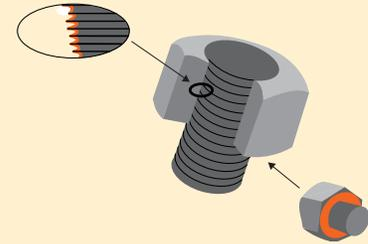
*Friction points should always be lubricated when using the torque tightening method.*
