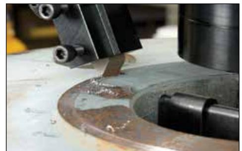
The Equalizer range of patented flange spreading tools have been developed to aid and simplify the maintenance of flange joints. No longer will those tasked with separating flanges have to rely on using ropes and pulleys, podgers, tirsors, come-alongs or hammers – there is a safe, quick and effective alternative, the Equalizer range of
