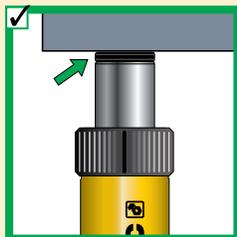
◀ Do not use cylinder without saddle. This will cause plunger to "mushroom". Saddles distribute load evenly on the plunger.
