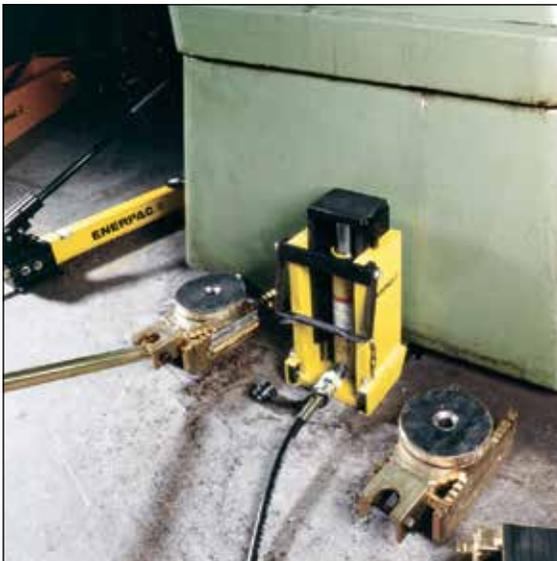
▼ Chemical tank transportation: The first inch(s) the load was lifted with an RCS-Series Low Height Cylinder and then moved onto load skates for transportation.
