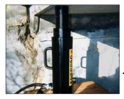
The portable Lock Nut cylinder RACL1506 used for extended load support during epoxy injection for bridge reinforcement.
