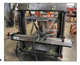
I-Beam end face milling with a GMRF1000. ▶
