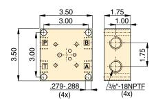
**Modular Valve Remote Mount Manifold**
