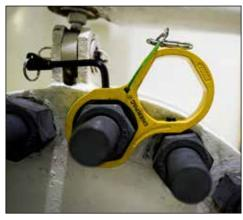
**▼** Shown: STTLS Safe T<sup>™</sup> Torque Lock
