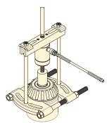
▲ Cross Puller with Bearing Separator on application
