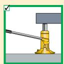
The entire jack saddle must be in contact with the load. Movement of the load must be in the same direction as jack plunger.
