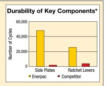
\*Average test results, whereby three Enerpac 1<sup>13</sup>/<sub>16</sub>" UltraSlim cassettes and three competitor 1<sup>13</sup>/<sub>16</sub>" cassettes were tested at 4000 ft-lbs for 50,000 cycles. The Enerpac side plates never broke for the full duration of the test.
