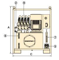
■ SFP-Series with 40-gallon reservoir (shown with 4 splitflow outlets)
