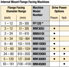
FF120 is not suitable for lens-ring flanges or ring type joints (RTJ) flanges.
