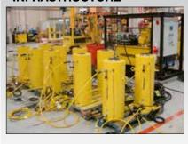
Custom cylinders with embedded sensors for bridge construction.
