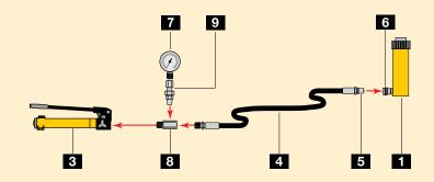
Single-acting cylinder with longer stroke used for lifting applications.
