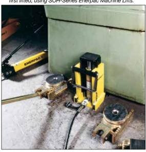
▼ Chemical tank transportation: The first inch(s) the load was lifted with an RCS-Series Low Height Cylinder and then moved onto load skates for transportation.
