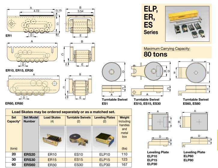
Sets are designed to enable two skates to take full load for extra safety on uneven floor surfaces
