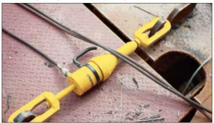
To lift a load bearing mast into place, BRP cylinders were used to tension the supporting cables.
