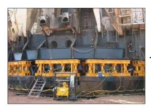
■ To prevent back pressure and to increase cylinder retraction speed, when using long hoses, the Enerpac HC7300 range of hoses with increased internal diameter is the best choice.
