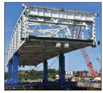
▼ Undecking an 1500-ton Electric Rope Shovel in a Copper Mine with a JS500 Jack-Up System for bearing inspection and maintenance.
