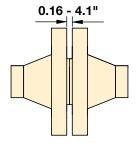
An innovative flange spreading wedge for use on small, medium or large flange joints with a minimum access gap of 0.16 inch. The SWi range includes ATEX approved options.
