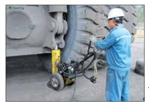
◆ Enerpac POW'R-RISER® used in mining operations to lift heavy equipment.
