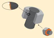
Friction points should always be lubricated when using the torque tightening method.
