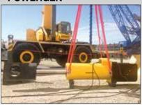
◆ One of three custom SyncHoist cylinders used to place a 1,140-ton nuclear plant module.
