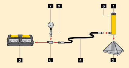
**Double-acting cylinder set-up** used for lifting applications where a slow controlled descent of the load must be maintained.
