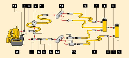
Two point lifting set-up using single-acting cylinders.
