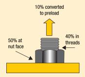
Frictional Losses (dry steel bolt)
